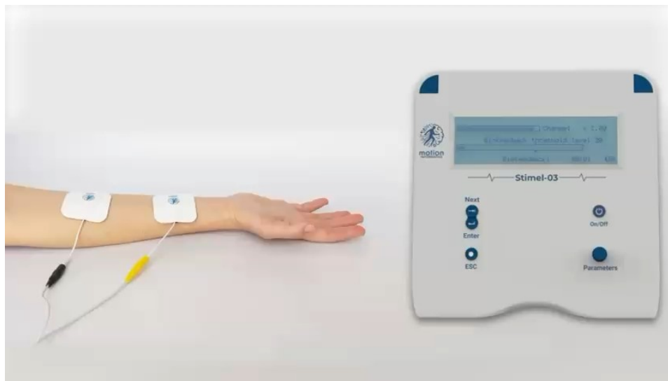
Figure 1. EMG Biofeedback Signal Detection Surface EMG electrodes detect electrical activity generated by muscle fibers during voluntary contraction. The signal is processed and displayed as visual biofeedback, allowing patients and clinicians to observe neuromuscular activation in real time.
